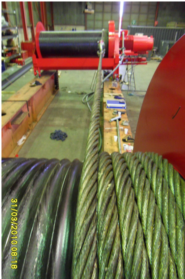
Winches on test bank, pulling test
